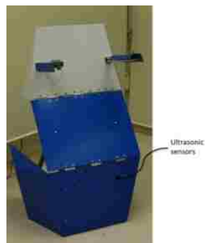
Figure 42 - Chair's ultrasonic sensors
